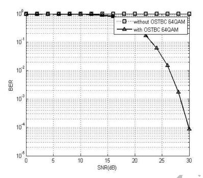
Fig. 6: BER comparison for 64-QAM
