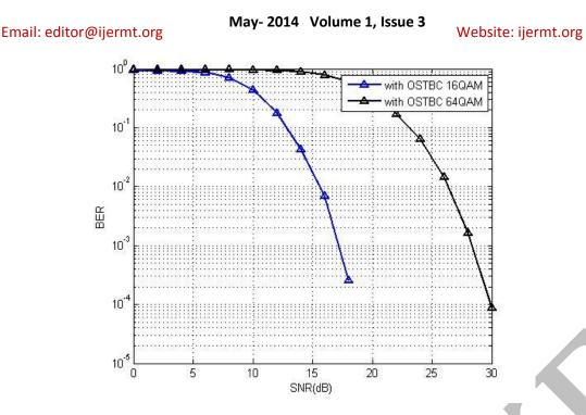
Fig.7: BER comparison of 16 QAM and 64 QAM for OSTBC
