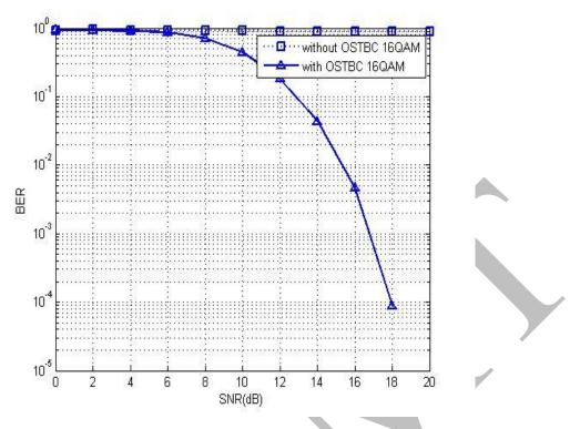
Fig. 5: BER comparison for 16-QAM
