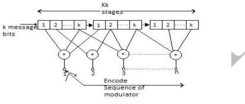
Fig. 3: Convolutional Encoder
